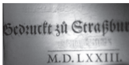
Light from infrared torch Note red print removed from view and indentions showing
